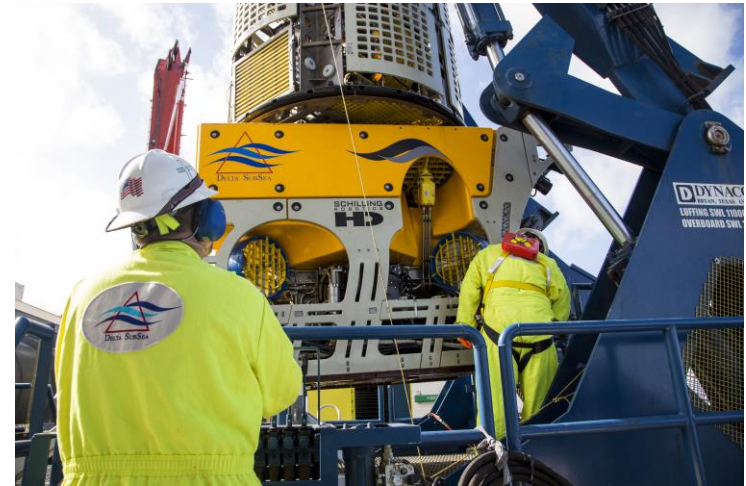
DSS pilot techs deploying HD-29 ROV
